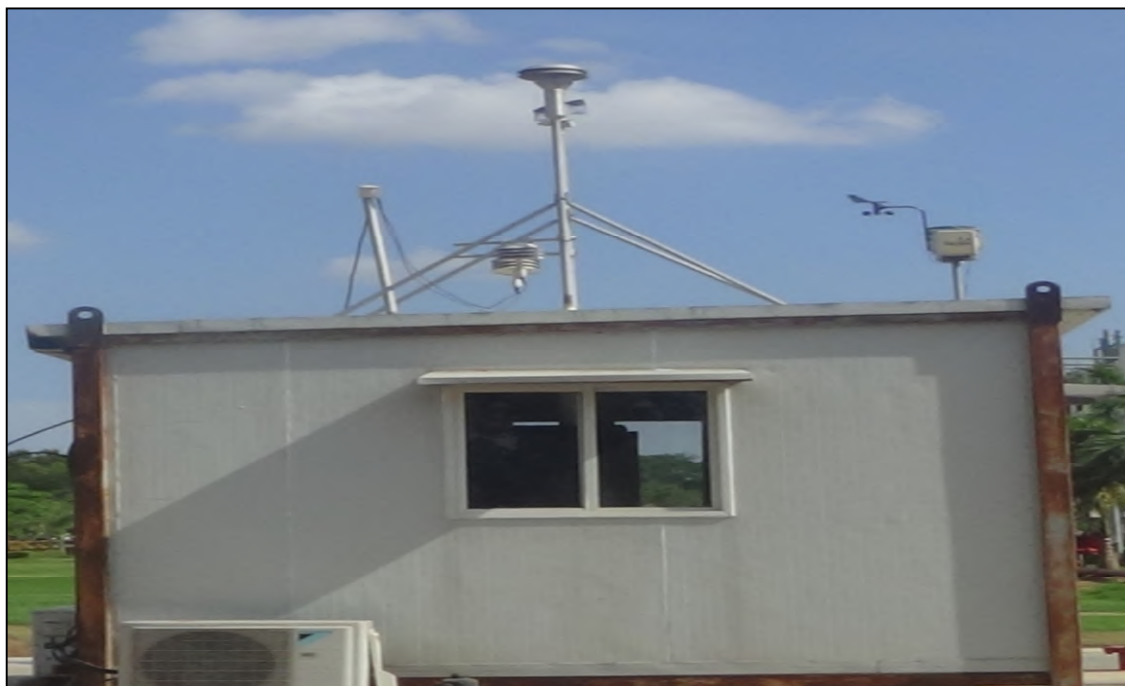
(A) Ambient Air Monitoring Station
